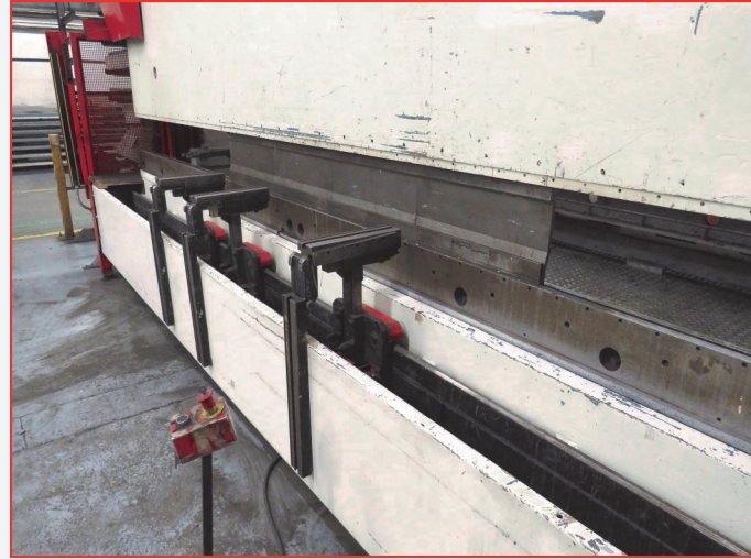
• Edwards Pearson PR10 250 Ton x 5100mm Over Bed CNC Press Brake, Admitting 4500mm Between Side Frames, 3000mm Long Heavy Duty Back Gauge with Cybelec DNC 800 8 Axis Control, Auto Crowing, Infra-Red Operator Guards, Hydraulic Top Tool Clamping, Side & Rear Safety Fences, Tooling Carousel (1997)
