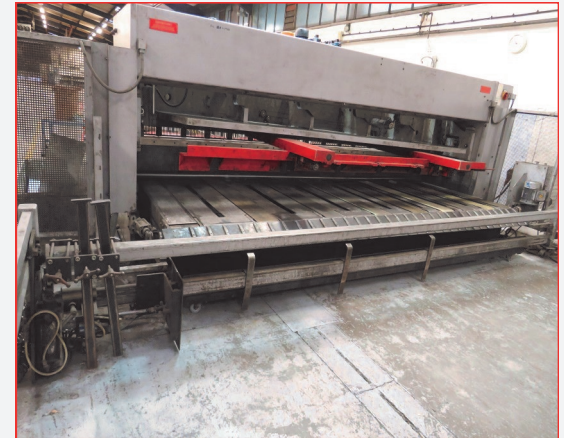
•Edwards Pearson VR 4080mm x 10mm Capacity Hydraulic Variable Rake Guillotine with Cybelelec DNC 10 Control, Auto Blade Gap Adjustment, Heavy Duty Rear Sheet Support System with Integrated Conveyor, (1) x 4000mm Squaring Arm, 3 x 2000mm Sheet Supports, Rear Infra-Red Safety Guarding (1997)
