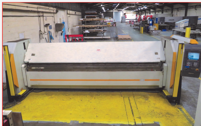
• RAS Type 73.40 Flexibend 4000mm x 2.5mm Capacity High Speed CNC Folder with System 5000 CNC Control System, 'J' Shape Back Gauge with 4000mm Reach, Max Bending Angle 180 deg, Full Length Segmented Goats Foot Top Tooling, (2) x Sets of Segmented Bottom Tools, Infra-Red Operator Guarding (2001)
