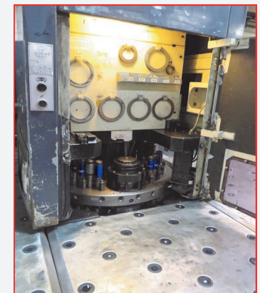
•LVD Delta 1250 Long Beam 20 Ton Capacity CNC Turret Punch with LVD MNC 32000 Control, Punching Area: 1250 x 2500mm or 1250 x 5000mm, Axis Travel: 1275 x 2525mm, 22 Station Thick Turret Configuration with (2) x 88.9mm Auto Index Stations, (3) x Programmable Sheet Clamps (1998)
