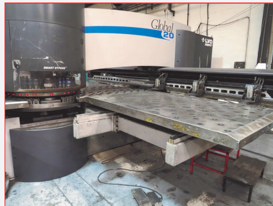
•LVD Strippit Global 20 Ton Capacity CNC Turret Punch with Fanuc 180i-PB Control, Punching Area: 1250mm x 2500mm or 1250mm x 5000mm, Axis Travel: 1275mm x 2525mm, 30-Station Thick Turret Configuration with (3) x 88.9mm Auto Index Stations, (3) x Programmable Sheet Clamps (2001)
