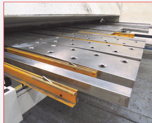
• RAS Type 73.40 Flexibend 4000mm x 2.5mm Capacity High Speed CNC Folder with System 5000 CNC Control System, 'J' Shape Back Gauge with 4000mm Reach, Max Bending Angle 180 deg, Full Length Segmented Goats Foot Top Tooling, (2) x Sets of Segmented Bottom Tools, Infra-Red Operator Guarding (2001)
