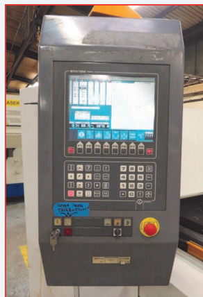
• RAS Type 73.40 Flexibend 4000mm x 2.5mm Capacity High Speed CNC Folder with System 5000 CNC Control System, 'J' Shape Back Gauge with 4000mm Reach, Max Bending Angle 180 deg, Full Length Segmented Goats Foot Top Tooling, (2) x Sets of Segmented Bottom Tools, Infra-Red Operator Guarding (2001)
