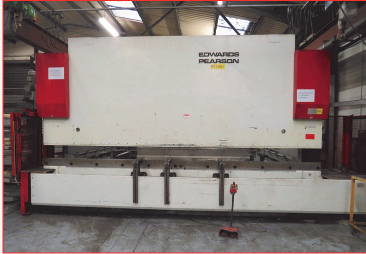
• Edwards Pearson PR10 250 Ton x 5100mm Over Bed CNC Press Brake, Admitting 4500mm Between Side Frames, 3000mm Long Heavy Duty Back Gauge with Cybelec DNC 800 8 Axis Control, Auto Crowing, Infra-Red Operator Guards, Hydraulic Top Tool Clamping, Side & Rear Safety Fences, Tooling Carousel (1997)
