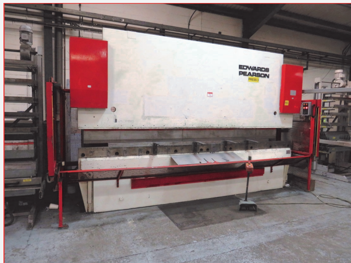
• Edwards Pearson PR6 150 Ton x 4100mm Over Bed CNC Press Brake with Cybelec DNC 880 6 Axis Control, (Y1, Y2, X, Z1, Z2, R) Auto Crowing, Infra-Red Guards, Hydraulic Top Tool Clamping, Side & Rear Safety Fences, Tooling Carousel (1999)
