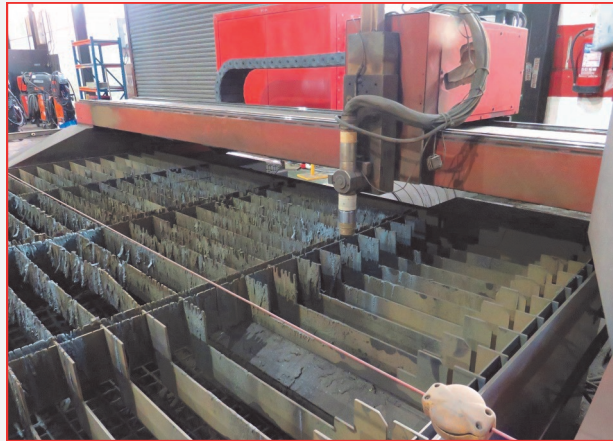
• Esprit Viper 3000 CNC Plasma Cutting Machine, 12m x 3m Table (Can be reduced in 2m long sections) with Hypertherm HPR 260 Power Source, Esprit Edge Pro CNC Control, PC & Software, Power Pierce Technology, Stand Alone Dust Extraction (2007)
