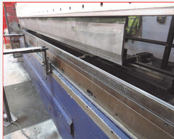
• Bystronic PR 150 Ton x 4100mm Over Bed CNC Press Brake with Cybelec DNC 1200 6 Axis Control, Auto Crowing, Laser Guards, Hydraulic Top Tool Clamping, Side and Rear safety Fences, Tooling Carousel (2004)
