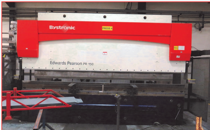
• Bystronic PR 150 Ton x 4100mm Over Bed CNC Press Brake with Cybelec DNC 1200 6 Axis Control, Auto Crowing, Laser Guards, Hydraulic Top Tool Clamping, Side and Rear safety Fences, Tooling Carousel (2004)
