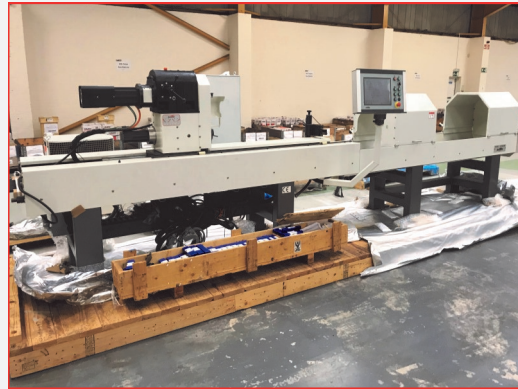
•2-off Sunnen Model HTC 2300W CNC Horizontal Hydraulic Hones (2009/2012)
