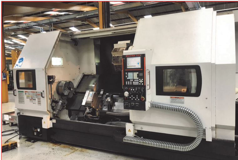
• Mazak Slanturn 50NR CNC Lathe with Mazatrol 640T CNC Control, 10-Position Turret, 2-Point Hydraulic Steady, Programmable Tailstock, 385mm 3-Jaw Hydraulic Chuck, Swarf Conveyor (05/2007)
