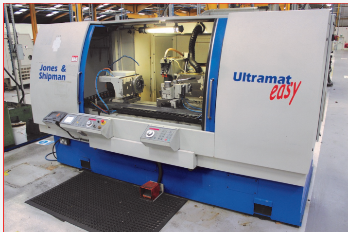
• Jones & Shipman Ultramat U1000 Easy-E CNC Cylindrical Grinder with GE Fanuc Control, Max. Swing: 320mm, Max Diameter Ground: 300mm (2007)
