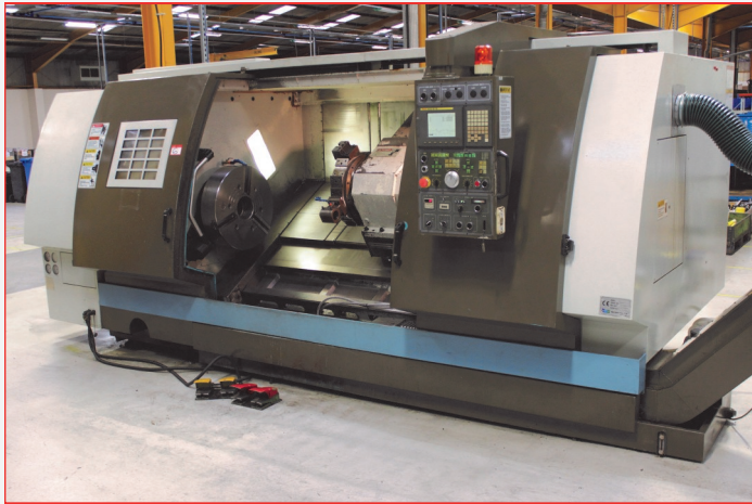
• Doosan 670L 2 Axis CNC Lathe with Fanuc 18i-TB CNC Control, 12 Position Turret, Tool Probing, 2-Point Hydraulic Steady, Swarf Conveyor (2005)
