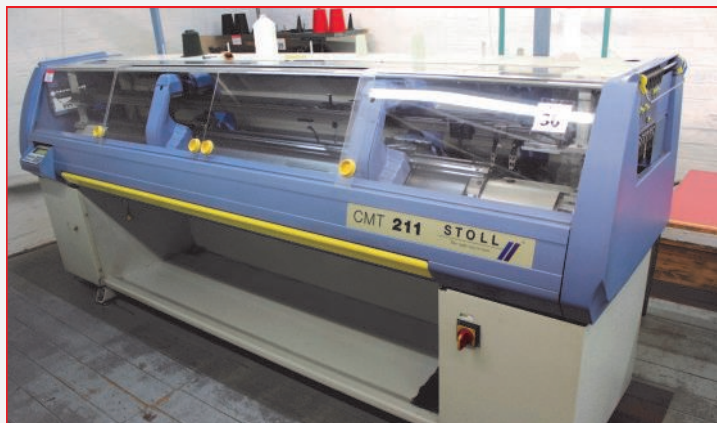
•Stoll CMT 211 450001 Computerised 10 Gauge Flatbed Knitting Machine
