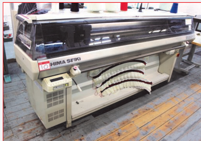
• Shima Seiki SFJ202-T Computerised 7 Gauge Flatbed Knitting Machine
