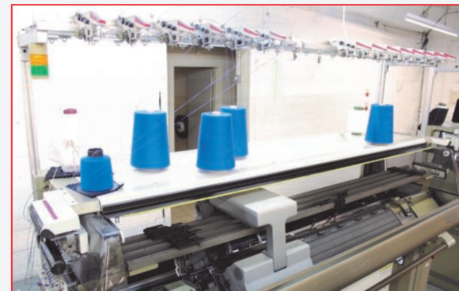
•(21) Shima Seiki SES122RT Computerised 10 Gauge Flatbed Knitting Machines (1995-1997)
