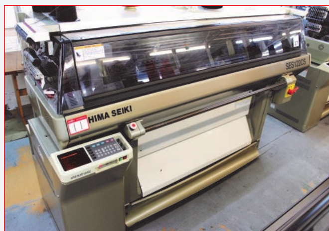
• Shima Seiki SES122CS Computerised 5 Gauge Flatbed Knitting Machine
