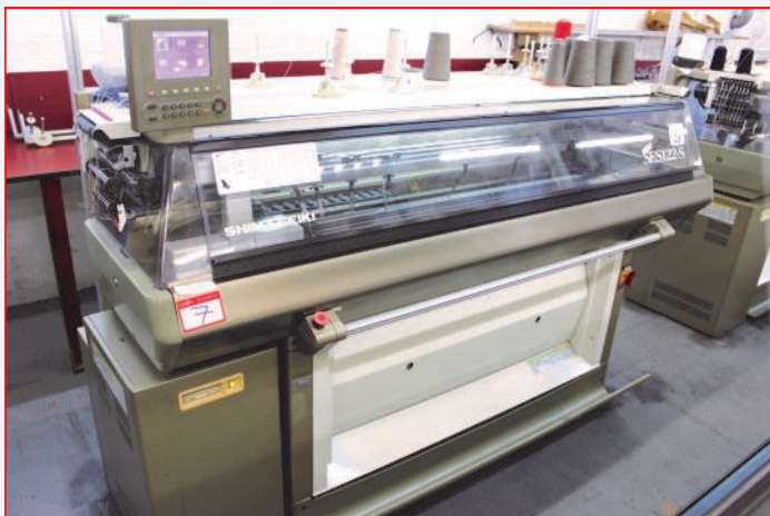
•(4) Shima Seiki SES122-S Computerised 7 Gauge Flatbed Knitting Machines (1995-2003)
