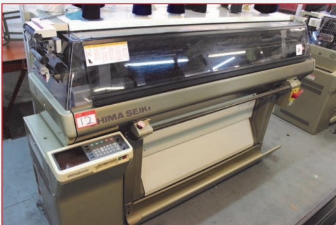
•(4) Shima Seiki SES122FF Computerised 7 Gauge Flatbed Knitting Machines
