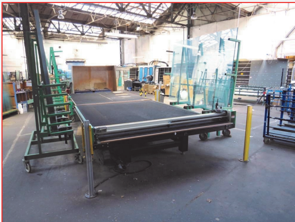
•MTL 3m x 2m XY Cutting Table, Model Panther ED with Edge Deletion, 3m x 2m Break Out Table, Break Out Bars & (2) Mobile Free Fall Racks (2012)
