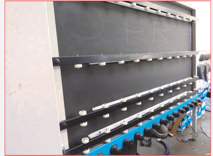
•Advanced Systems 1.6 Vertical Glass Washer, Manual In-feed Power Out-feed
