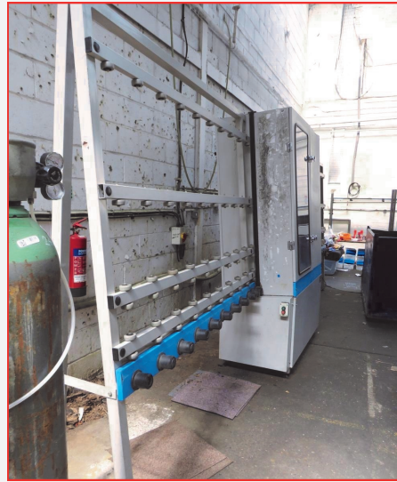
•Advanced Systems 1.6 Vertical Glass Washer, Manual In-feed Power Out-feed
