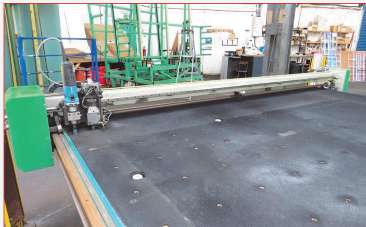
•MTL 3m x 2m XY Cutting Table, Model Panther ED with Edge Deletion, 3m x 2m Break Out Table, Break Out Bars & (2) Mobile Free Fall Racks (2012)
