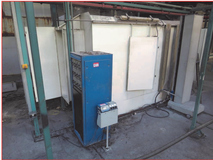
• Powder Coating Booth, Working Area 1.6m x 450mm
