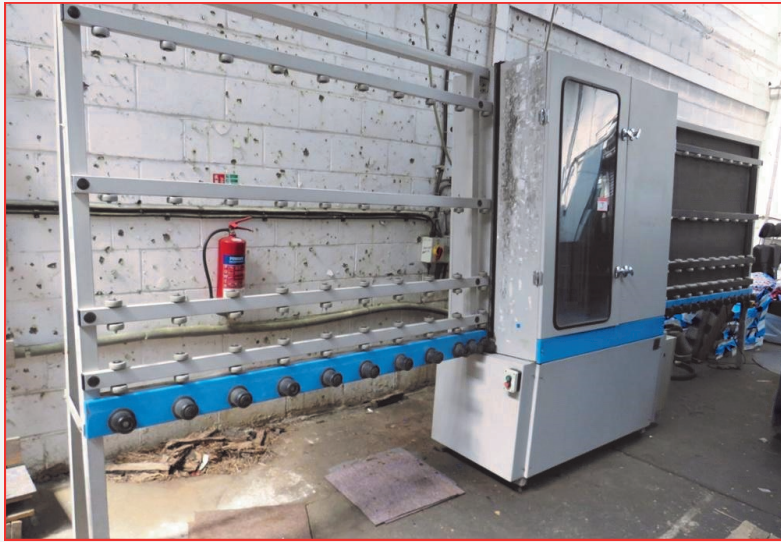
•Advanced Systems 1.6 Vertical Glass Washer, Manual In-feed Power Out-feed
