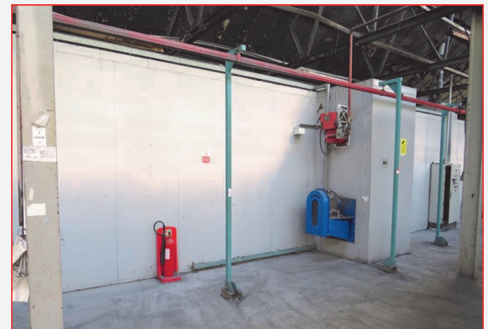
• Gas Fired Tunnel Oven for Paint Booth, Working Area 1.6m x 450mm
