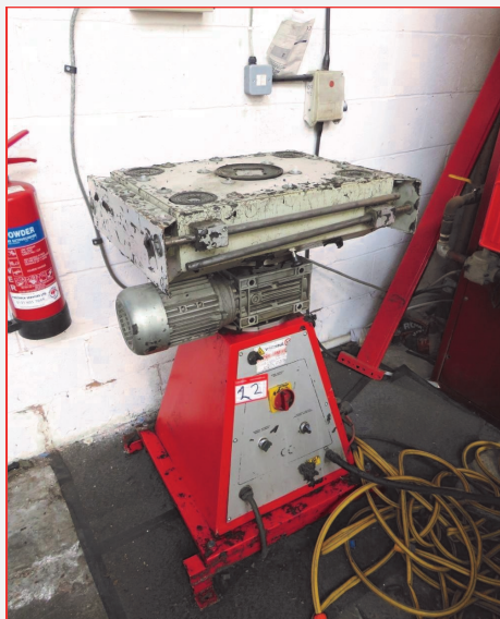
•Rotating Hot Melt Table Type M116 (1999)
