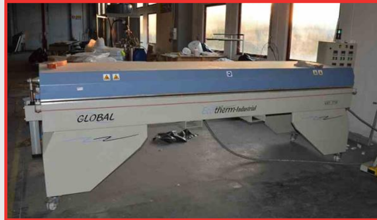
• Global Type GET 3710 Pre-Heating Oven for Acrylic Solid Surfaces, Dimensions: 3700 x 1000mm (2007)
