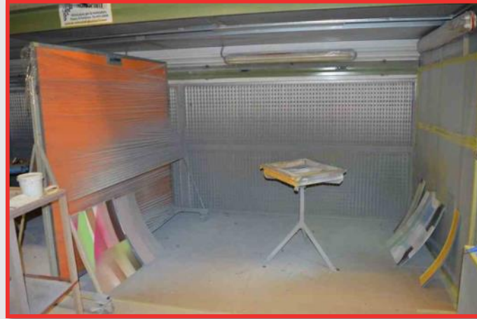
· (2) Pacini Type 1S52422SS Spray Booths; Dimensions 5500 x 2250 x 2000mm with Division Screen & Exhaust Trunking (2006)
