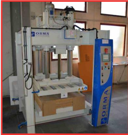
• Orma Machine PFS-5 DIGIT 03/12 Hydraulic Four Ram Cold Press (2013)
