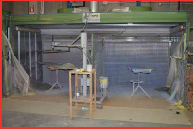
· (2) Pacini Type 1S52422SS Spray Booths; Dimensions 5500 x 2250 x 2000mm with Division Screen & Exhaust Trunking (2006)
