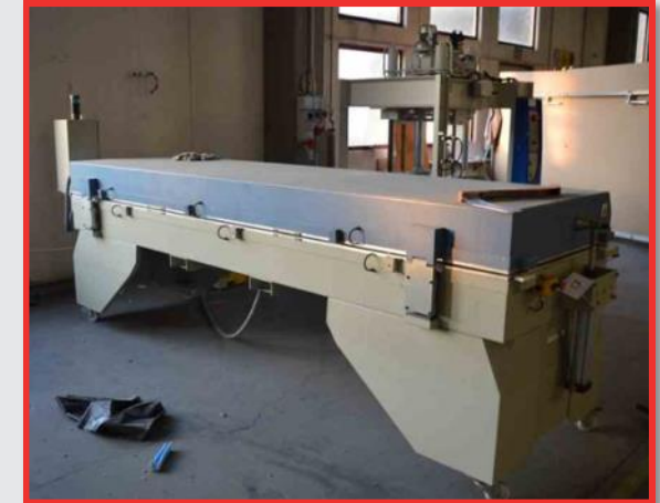
• Global Type GET 3710 Pre-Heating Oven for Acrylic Solid Surfaces, Dimensions: 3700 x 1000mm (2007)
