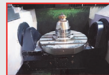
• (2) Doosan VC630/5AX 5-Axis Vertical Machining Centres with Heidenhain iTNC Controls, 60 Station Tool Changer, Table Size 600mm x 600mm (2014)
