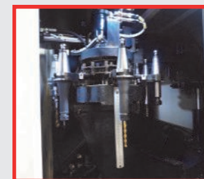
• (2) Doosan VC630/5AX 5-Axis Vertical Machining Centres with Heidenhain iTNC Controls, 60 Station Tool Changer, Table Size 600mm x 600mm (2014)
