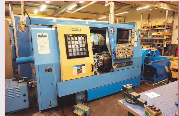
Mori Seiki ZL-15m Twin Turret CNC Lathe with Fanuc 11TT Control, 170mm 3-Jaw Chuck, 6 & 8-Station Tool Changers, Tailstock & Swarf Conveyor
