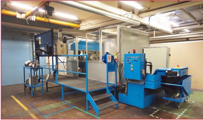
AB Korner MEK Verktast Borrautomat 4 Head Drilling and Turning Machine, Swarf Conveyor, 630mm 3 Jaw Chuck with various Face Plates, Knoll Coolant System (2003)
