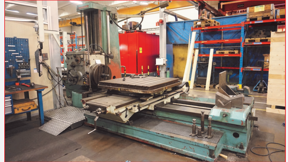
TOS Varnsdorf Vertical Borer, With Heidenhain D.R.O, Table size 1250mm x 1250mm, 50 International Tooling, 600mm Boring Face
