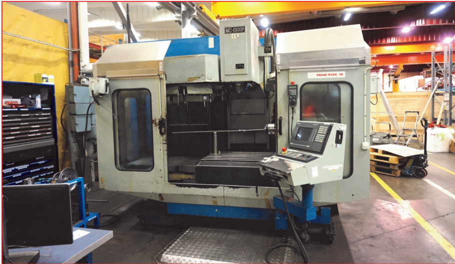
Fumac MC-1300P Vertical Machining Centre with Siemens Sinumerik Control, Table size 1.5m x 700mm, CAT40 Tooling, 30 Station ATC, Qty Tooling, Swarf Conveyor (7/1996)
