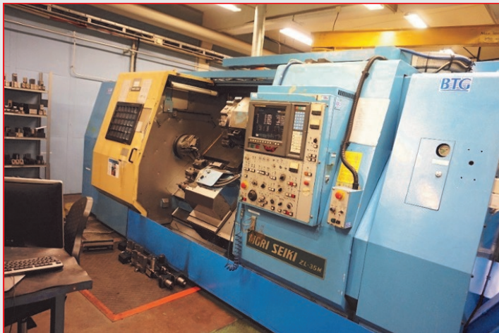
Mori Seiki ZL-35M Twin Turret CNC Lathe with Fanuc Series 15-TT Control, 315mm 3-Jaw Chuck, 10 & 12-Station Turrets, Swarf Conveyor & Tailstock (12/1996)
