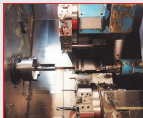
Mori Seiki ZL-15m Twin Turret CNC Lathe with Fanuc 11TT Control, 170mm 3-Jaw Chuck, 6 & 8-Station Tool Changers, Tailstock & Swarf Conveyor
