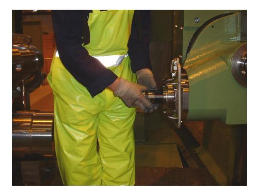
➢ Assemble the Capto end plate.
