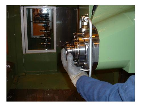
➤ Tighten in place 14-off cap screws stamped 12.9.
