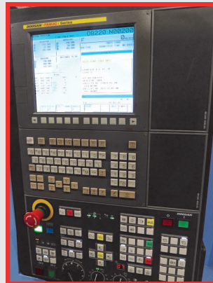
• (2) Doosan Lynx 220LM Compact Multi Axis CNC Turning Centres with Fanuc i Series Control, 'C' Axis and Driven Tools, 24-Station Turret, Bar Capacity: 51mm, 6" Chuck, Max. Workpiece: 500mm, Toolsetter, Parts Catcher, Tooling Package with 4 Driven Tools: 2 Axial and 2 Radial (2014)
