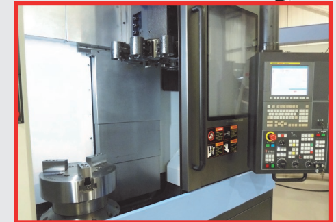
• Doosan Puma VT750 Vertical 2-Axis CNC Lathe with Fanuc i Series Control, Renishaw Probe, 18" Chuck, Max. Workpiece Height: 750mm, Tooling Package (2014)
