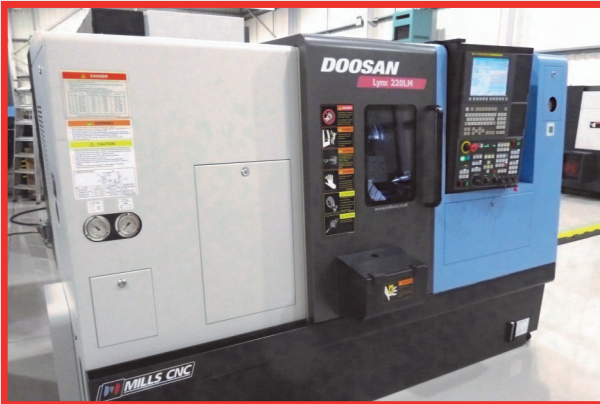
• (2) Doosan Lynx 220LM Compact Multi Axis CNC Turning Centres with Fanuc i Series Control, 'C' Axis and Driven Tools, 24-Station Turret, Bar Capacity: 51mm, 6" Chuck, Max. Workpiece: 500mm, Toolsetter, Parts Catcher, Tooling Package with 4 Driven Tools: 2 Axial and 2 Radial (2014)
