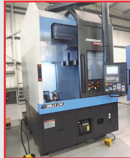
• Doosan Puma VT750 Vertical 2-Axis CNC Lathe with Fanuc i Series Control, Renishaw Probe, 18" Chuck, Max. Workpiece Height: 750mm, Tooling Package (2014)
