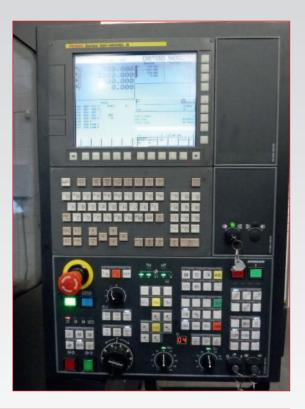
• **DOOSAN Puma** 700LY Heavy Duty CNC Turning Centre with Fanuc 32i Control, 'Y' Axis, 'C' Axis and Driven Tools, 3200mm between Centres, Bar Capacity: 164mm, Toolsetter, Programmable Tailstock, 45kw Main Spindle Drive, Tooling Package with 4 Driven Tools: 2 Axial and 2 Radial (2014)
