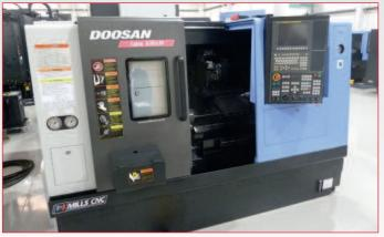
• (2) Doosan Lynx 220LM Compact Multi Axis CNC Turning Centres with Fanuc i Series Control, 'C' Axis and Driven Tools, 24-Station Turret, Bar Capacity: 51mm, 6" Chuck, Toolsetter,
