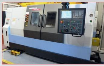
Doosan Puma 400MB 2-Axis Heavy Duty CNC Turning Centre with Fanuc 32i Control, 'C' Axis and Driven Tools, 1050mm between
