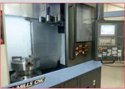
DOOSAN Puma VT750 Vertical 2-Axis CNC Lathe with Fanuc i Series Control, Renishaw Probe, 18" Chuck, Max. Workpiece Height: 750mm, Tooling Package (2014)
