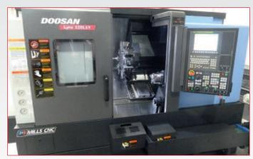
• Doosan Lynx 220LSYA Compact Multi Axis CNC Turning Centre with Fanuc i Series Control, 'Y' Axis, 5" Sub-Spindle, 'C' Axis and Driven Tools, 24-Station Turret, Bar Capacity: 51mm, 6" Chuck, Toolsetter, Parts Catcher, Parts Conveyor, Tooling Package with 4 Driven Tools: 2 Axial and 2 Radial (2014)
