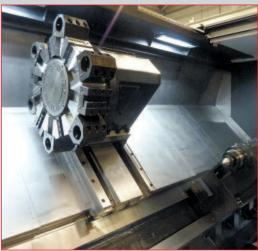
• **DOOSAN Puma** 700L Heavy Duty CNC Turning Centre with Fanuc 32i Control, 3200mm between Centres, Bar Capacity: 164mm, Toolsetter, Programmable Tailstock, 45kw Main Spindle Drive, Tooling Package (2014)
