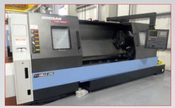
Doosan Puma 400LMB Heavy Duty CNC Turning Centre with Fanuc
