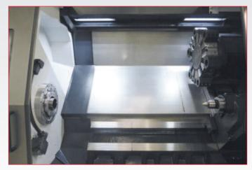
• **DOOSAN Puma** 600 Heavy Duty CNC Turning Centre with Fanuc 32i Control , 1600mm between Centres, Bar Capacity: 116mm, Toolsetter, Programmable Tailstock, 37kw Main Spindle Drive, Tooling Package (2014)
