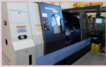
Doosan Puma 400B 2-Axis Heavy Duty CNC Turning Centre with Fanuc 32i Control, 1050mm between Centres, Bar Capacity: 116mm, 15" Chuck, Toolsetter, Programmable Tailstock, 22kw Main Spindle Drive, Tooling Package (2014)
