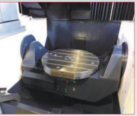
• DOOSAN Puma VC630-5AX 5-Axis CNC Vertical Machining Centre with Heidenhain 530i Control, 60-ATC, 40 International Taper, 630mm x 590mm Table, Traverses: X = 650mm, Y= 765mm, Z = 520mm, Through Spindle Coolant (2014)
