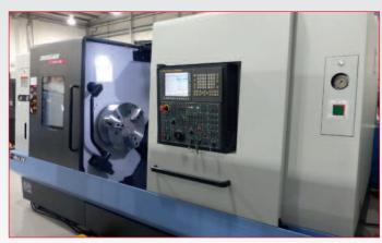
• (2) Doosan Puma 480 2-Axis Heavy Duty CNC Turning Centres with Fanuc 32i Control, 1000mm between Centres, Bar Capacity: 165mm, 21" Chuck, Toolsetter, Programmable Tailstock, 45 kw Main Spindle Drive, Tooling Package (2014)
